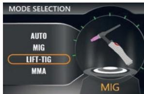
The TIG method is especially recommended for aesthetic and high-quality metal welding, without labour-intensive machining afterwards. However, this requires proper preparation and cleaning of the edges of both welded pieces. Mechanical properties of the additional material should be similar to those of the welded pieces. The shielding gas is pure argon, supplied in the amount according to the welding current settings.
